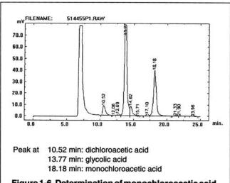
Figure 1-6. Determination of monochloroacetic acid, dichloroacetic acid and glycolic acid by HPLC
