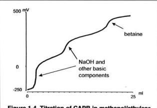
Figure 1-4. Titration of CAPB in methanol/ethylene glycol menomethyl ether with perchloric acid in dioxane
